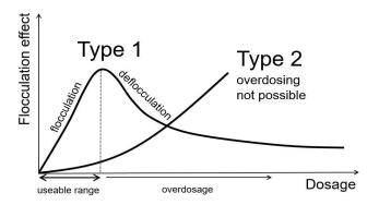
Fig. 2. Simplified diagram of flocculation effect vs. dosage for the two types
